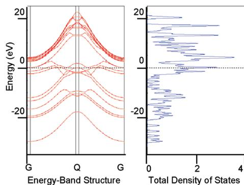
**Figure 7.** Electronic structure of the cell used to generate a 3-D array of  $C_3H_3$  with  $a = b = 20$  Å and  $c = 1.35$  Å. The energy-band structure on the left is measured from the Fermi energy level (dotted line) and plotted along the  $c$ -direction of the cell in reciprocal space; the corresponding total DOS is plotted on the right.
