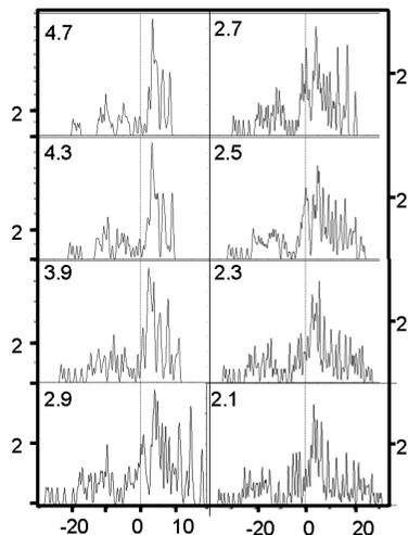
**Figure 8.** DOS of  $C_3H_3$  units in a linear array with different cell sizes (fixed  $a = 20$ ,  $b = 20$ , and  $c$  ranging from 2.1 to 4.7 Å). The horizontal-axis is the energy level and the vertical axis is the DOS. The dotted line indicates the Fermi level.
