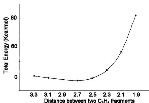
**Figure 2.** Total energy vs distance between two  $C_3H_3$  molecules. The energy stabilizes slowly before 2.7 Å and rises up rapidly when the distance of two  $C_3H_3$  molecules further decreases.
