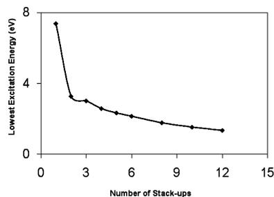
**Figure 5.** TD-DFT simulation of the lowest excitation energy of  $C_3H_3$  molecules in a linear array was limited to 12 molecules due to computational cost. Calculations were carried out by Gaussian 03 using 6-31++G(d',p') with the B3LYP method.
